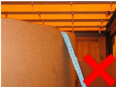
Figure 34. Example of a damaged reel edge
