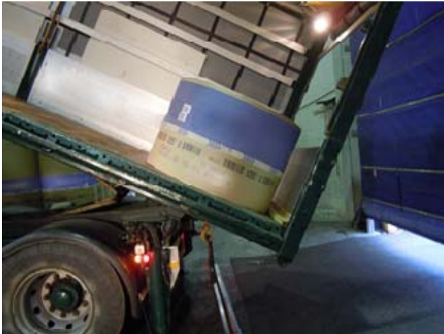
7a. Inclination test for determination of the friction between the reel and the platform floor
