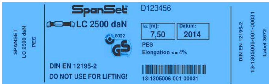
Figure 2. Typical content of webbing strap label, marked in accordance with EN 12195-2
